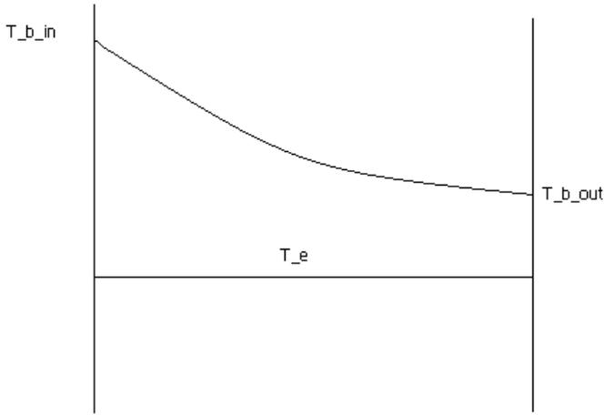
Figure 15: Temperature variation in evaporator
