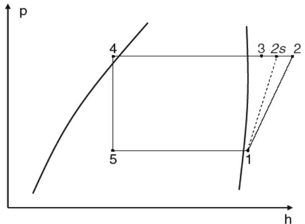
Figure 14: T-h diagram of Vapor compression cycle
