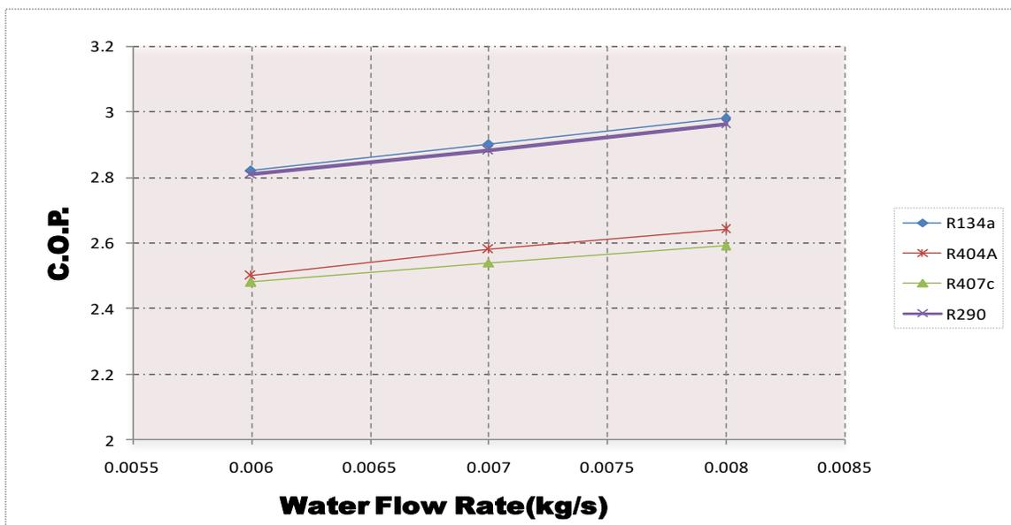
Figure 18: Variation of C.O.P with condensing water flow rate of VCRES using different refrigerants
