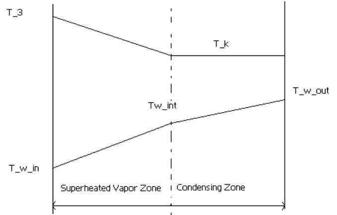
Figure 16: Temperature variation in condenser
