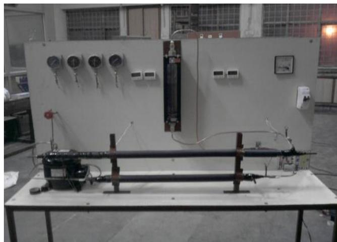
Figure 1: Vapour compression refrigeration system model
