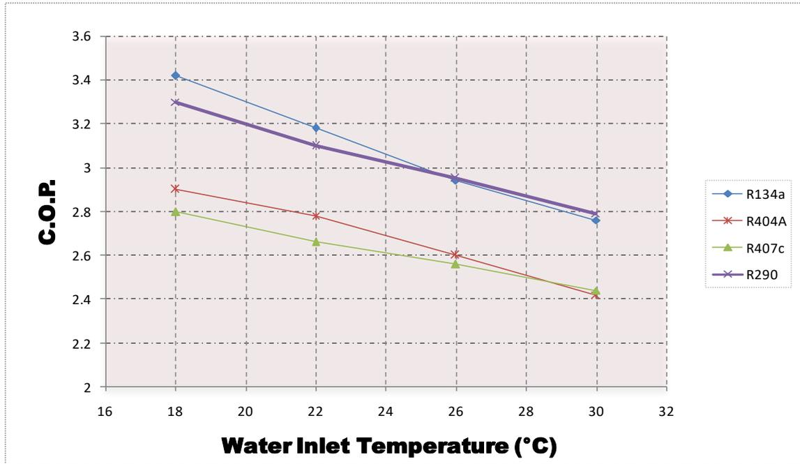
Figure 19: Variation of C.O.P with condensing water inlet temperature of VCERS using different refrigerants
