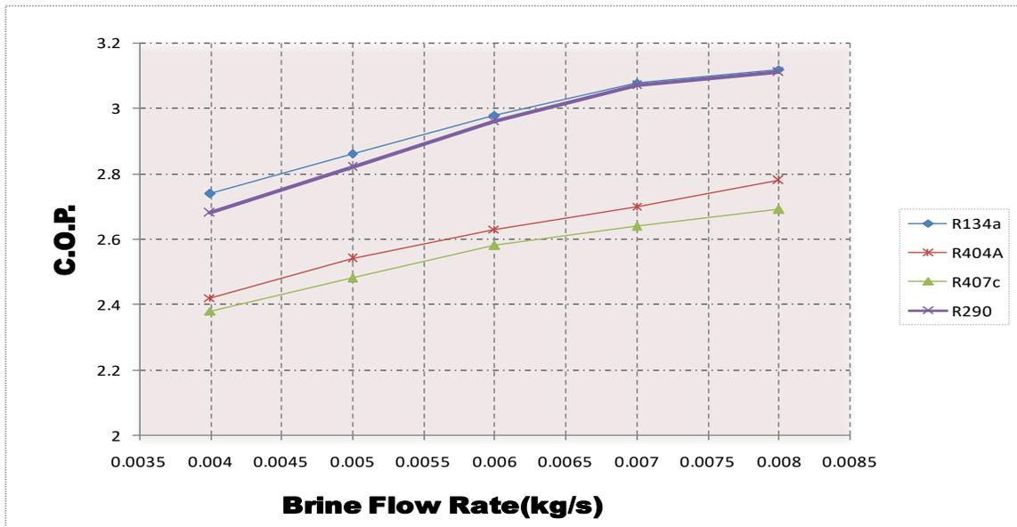
Figure 17: Variation of C.O.P with brine flow rate of VCRES using different refrigerants
