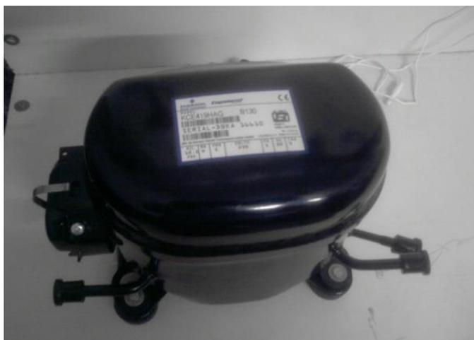
Figure 2: Hermetically sealed reciprocating compressor
