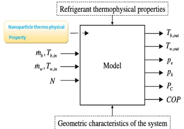
Figure 12: Vapour compression refrigeration system Model
