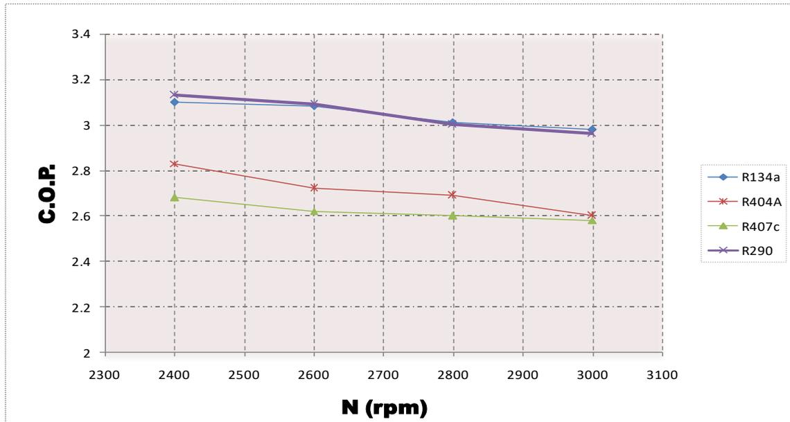
Figure 21: Variation of C.O.P. with Compressor speed of VCRS using different refrigerants
