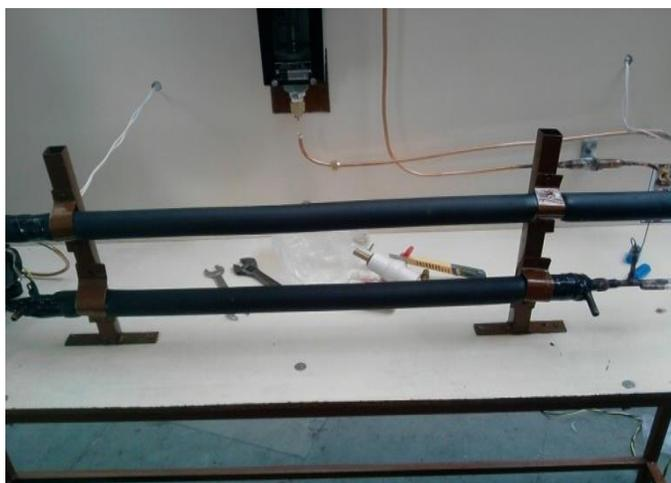
Figure 10: Condenser and evaporator
