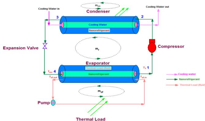
Figure 13: Schematic diagram of vapour compression refrigeration system model
