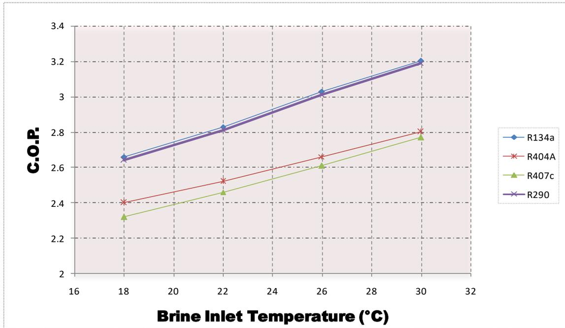
Figure 20: Variation of C.O.P with Brine inlet temperature of VCERS using different refrigerants
